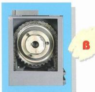
A torque limiter is provided to slip in the event of overload or blockage so as to protect motor and feed chain.
